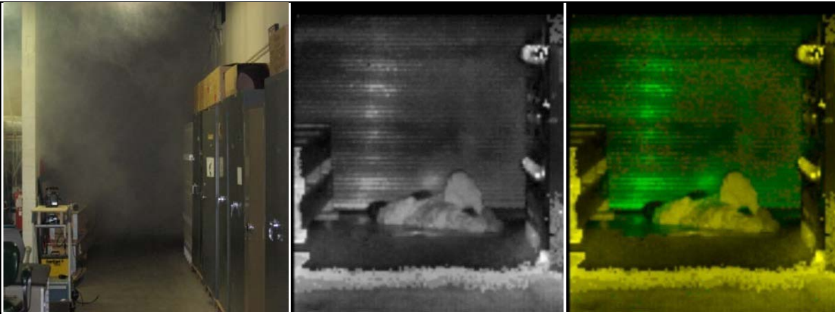
a) b) c) Figure 3. ASC's 3D camera can penetrate smoke to return 3D images in real-time a) Visible image of smoke filled room taken with a digital camera. b) 2D intensity image taken with ASC's 3D camera in smoke penetration mode. c) ASC's camera returns range and intensity of objects in the smoke cloud. Image is color encoded for range Data 2008 Used by permission from Applied Research Laboratory, Penn State University
