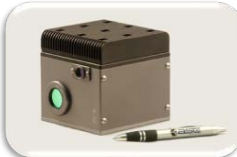
Figure 4a. Shibuya Street Scene Figure 4b. TigerEye with 45-degree Lens (11.2 cm x 12.2 cm x 11.9 cm; 1.87 kg)
